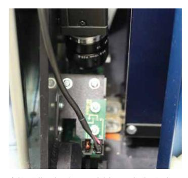
An integrated barcode reader scans cards during processing, time stamping each record, maintaining an unbroken chain of custody and ensuring complete dosimeter data tracking.
