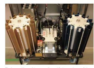
Simple menu driven maintenance routines and features such as small clean out drawers for inspecting and cleaning of the photo multiplier tubes, easily removable covers to access internal parts without disconnection, and a slide-mounted transport mechanism to access moving parts, simplify maintenance to increase reader uptime. The Harshaw 8800Plus has the highest capacity and lowest MTBF in the market today.
