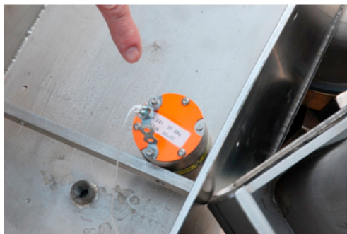
1 Ci Am-241 source in Tungsten shielding container
