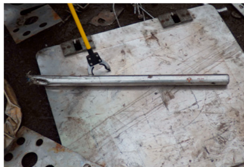
50 mCi AmBe industrial source found in steel scrap
