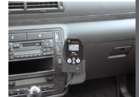
RadEye car adapter for mobile area survey applications
