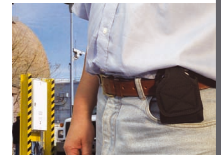
RadEye belt holster with openings for alarm-LED and earphone connector
